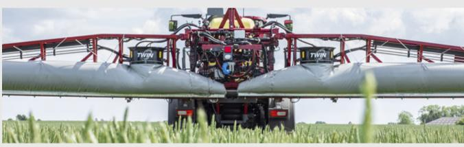
The Air-assisted TWIN FORCE boom employs the world's best system for spray control. Two powerful blower units provide air to the left and right boom sides.
