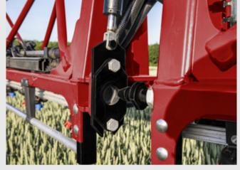
A stop-and-lock system avoids slack between the boom sections, which are folded and unfolded smoothly with SoftOpen/SoftClose.
