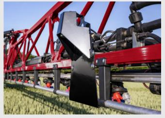
The unrivalled AutoTerrain boom management system uses advanced ultrasonic sensors to secure constant boom height. Works in either Soil Mode™, Crop Mode<sup>™</sup> or Hybrid Mode<sup>™</sup>.
